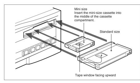
The cassette is automatically drawn into the unit and the tape is wound round the head drum. The tape is stationary while the head drum rotates, and the STOP button lights.
